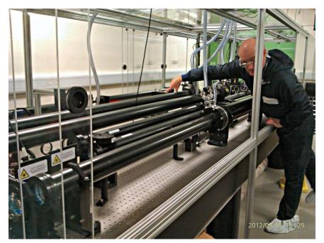
Astra is a high power, ultrashort pulse, high repetitionrate laser. It uses titaniumdoped sapphire (TiS) as its active material, and works at 800 nm in the near infra-red part of the spectrum, just outside the region visible to the human eye
