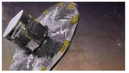
The camera used for this is one of the most advanced digital CCD (Charge Coupled Device) cameras in existence and is composed of an array of 106 CCDs with a resolution of around 1 billion pixels. Gaia orbits the Sun and in six hours the two telescopes within scan one large circle to observe around 10 million objects.
