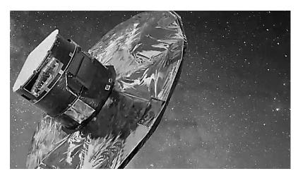
The camera used for this is one of the most advanced digital CCD (Charge Coupled Device) cameras in existence and is composed of an array of 106 CCDs with a resolution of around 1 billion pixels. Gaia orbits the Sun and in six hours the two telescopes within scan one large circle to observe around 10 million objects. These are not only stars but
