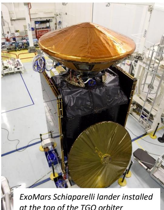
*ExoMars Schiaparelli lander installed at the top of the TGO orbiter*
