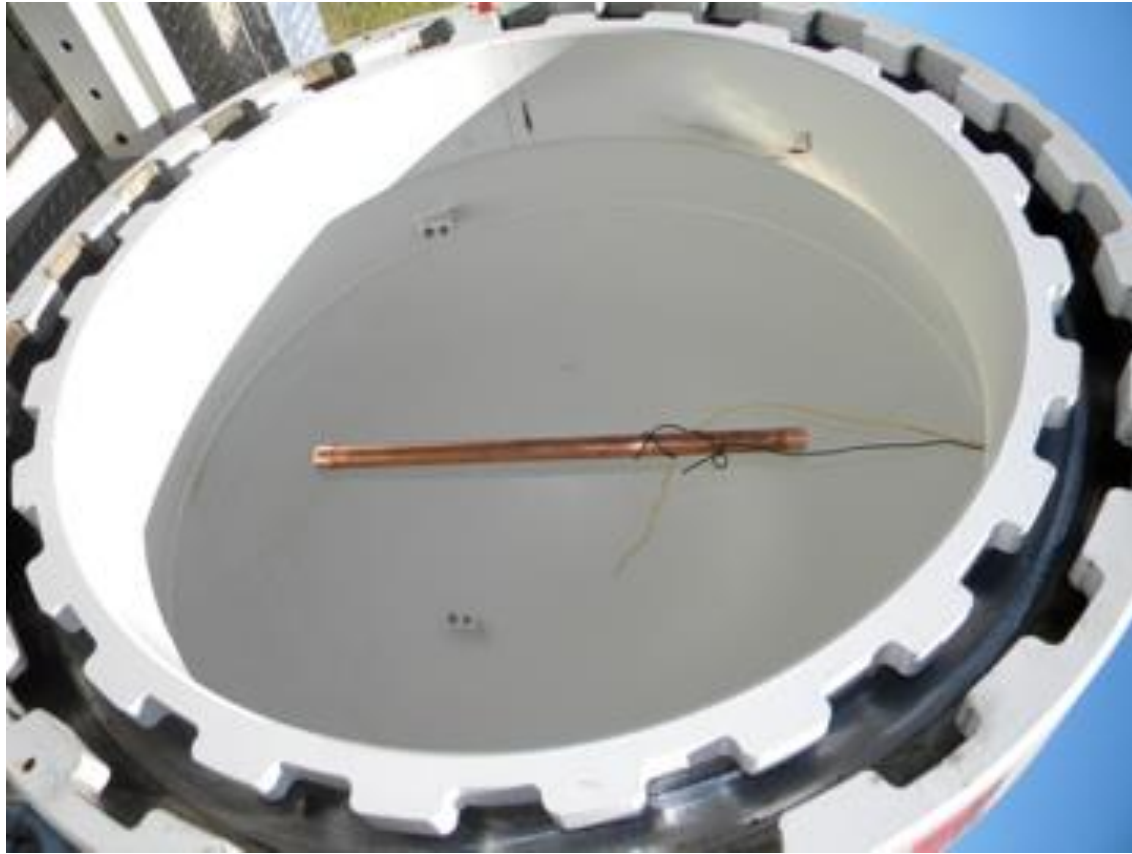
Dynasafe explosion containment vessel
