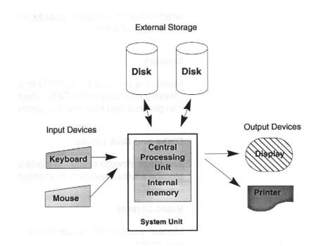
The term "computer" has also been loosely used to refer to the system unit. The system unit is composed of the following main components:
