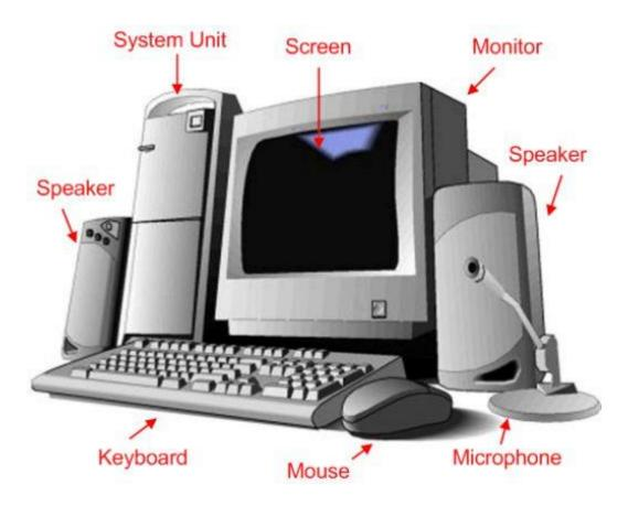
A computer is made up of four essential parts: the system unit, monitor, keyboard, and mouse. It would be very hard, if not impossible, to operate the computer if one of these were missing. You could, of course, still use the computer without a mouse if you memorized all the keyboard shortcuts, but the graphical nature of most programs nowadays has made the mouse an indispensable part of the computer.
